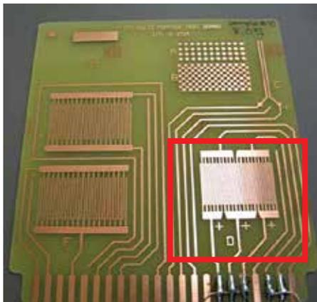
Figure 1. IPC-B-25A test vehicle used in this experiment.
