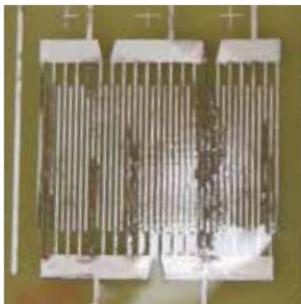
After 245 hours, severe corrosion was present on the control (uncoated).
